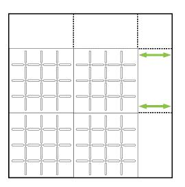
Border tiles are necessary around the edge of the ceiling when it is too small to accomodate full-size tiles. These edge trim tiles have been designed with a minimum relief pattern that lends itself to cutting and trimming.
