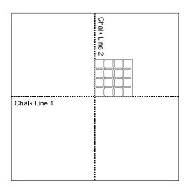
Taking into account the variables listed above, place chalk lines along the ceiling's midpoints. These lines should be parallel with the walls and create a cross close to the middle of the ceiling. These markings will help you align the edges of your first ceiling tiles.
