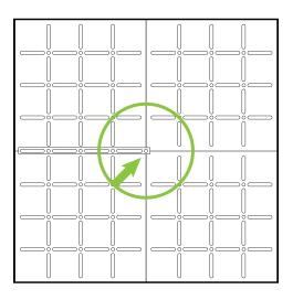
Do not remove the backing on decorative strips until they are ready to be installed, and make sure your ceiling tiles are clean and dry. If the adhesive on the back of the decorative strip comes into contact with dust, oil, or grease of any kind it will not adhere properly.
