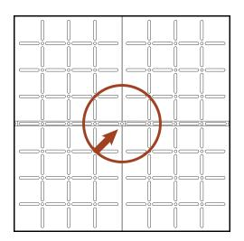
Remove the backing on the strip, exposing the adhesive, and press the strip firmly into place. Make sure to place the dot end of the strip over the intersection of four ceiling tiles and its length over the joint of two neighboring tiles.
