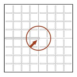
Do not remove the backing on decorative strips until they are ready to be installed, and make sure your ceiling tiles are clean and dry. If the adhesive on the back of the decorative strip comes into contact with dust, oil, or grease of any kind it will not adhere properly.
